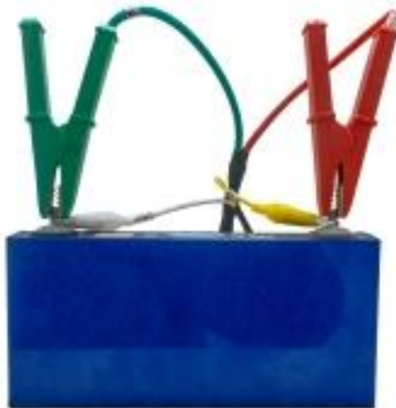
Connection of booster with battery core anode and cathode
